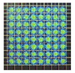
64 QAM signal with strong broadband noise. Possible cause: cable loss is to high or amplifier has a defect.
